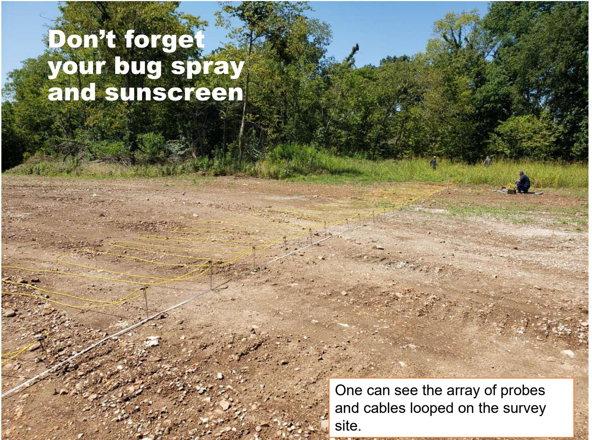
One can see the array of probes and cables looped on the survey site.
